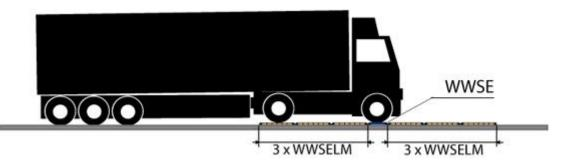
NOTE: The best condition of weighing is accomplished by creating a leveled area with a length equal to twice of the longest vehicle to be weighed.
